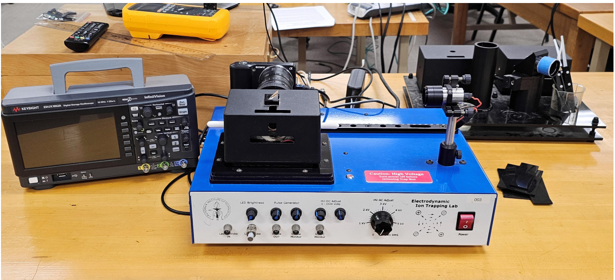
Figure 1. The Electrodynamic Ion Trapping experiment in the Ph3 lab. There are four such setups available.
