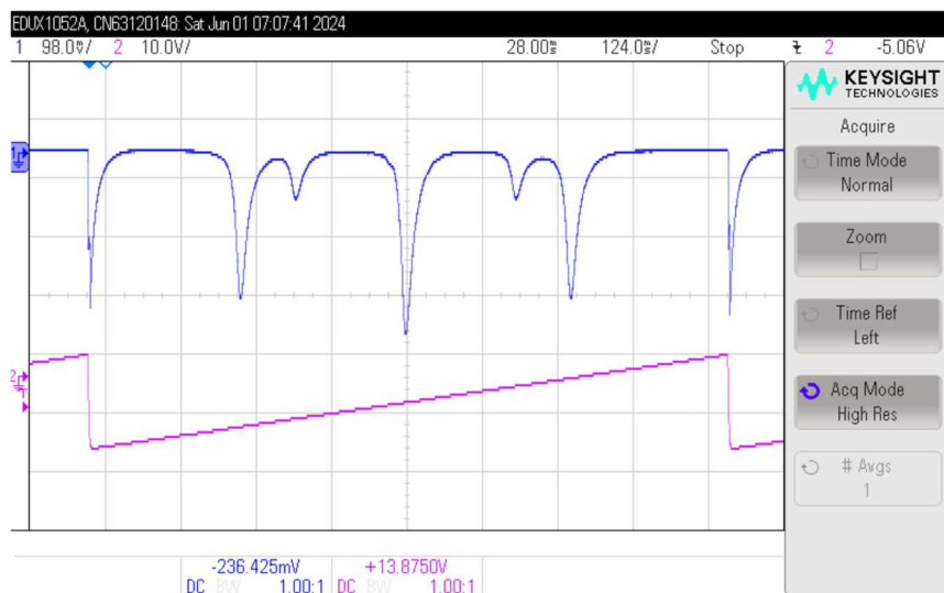
Figure 9. A typical oscilloscope screen once you have the 'scope triggering well with the optical-pumping signal placed nicely on the screen. The bottom trace (red) shows the linear ramp of axial magnetic field, with B = 0 at the center of the screen. The top trace shows the photodiode signal. Note that abrupt B -field transitions affect the photodiode amplifier electronics, and this produces spurious dips at these transitions.
