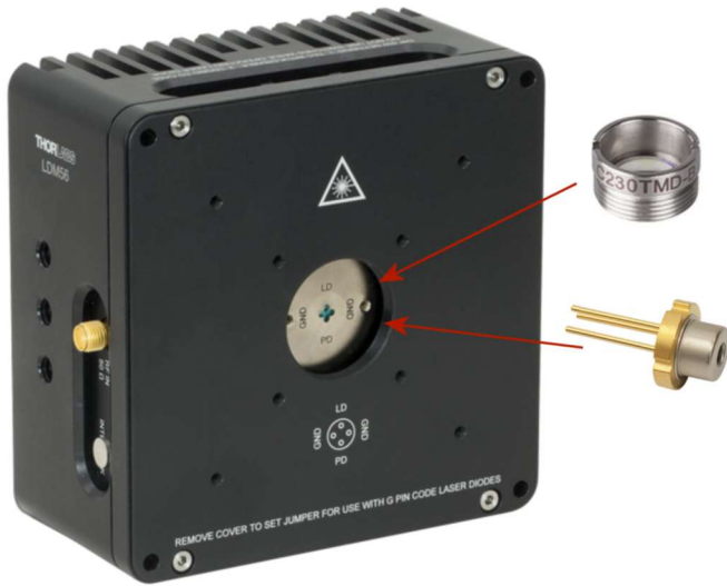
Figure 8. The LDM56 holds the diode laser can (lower right) and a collimating lens (upper right). The bulk of this unit is a large heat sink used for controlling the temperature of the diode laser.
