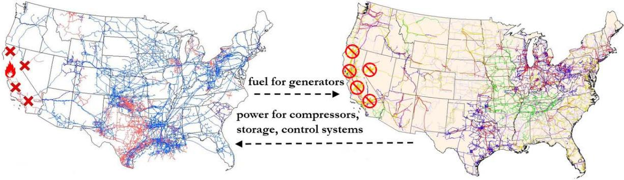
**Figure 2. Failure propagation in coupled infrastructure networks: U.S. natural gas pipeline network (on the left, source: Energy Information Administration) and U.S. power grid (on the right, source: <https://commons.wikimedia.org/wiki/File:UnitedStatesPowerGrid.jpg>).**
