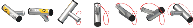
Fig. 14. Rotation about the intermediate inertial axis is unstable [Poincaré 1851] (see also [Landau and Lifshitz 1976, p. 118]), leading to periodic orientation changes. Our algorithm keeps angular momentum constant by construction which allows us to faithfully reproduce such instability phenomena. Here a single (half) cycle is shown with the intermediate axis marked as it traces out a 180^\circ turn. Video 3:40.
