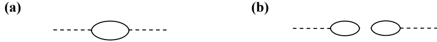
Fig. II.10.3 Second-order corrections to the phonon propagator: (a) connected polarization correction; (b) disconnected correction, which can be shown to vanish identically.
