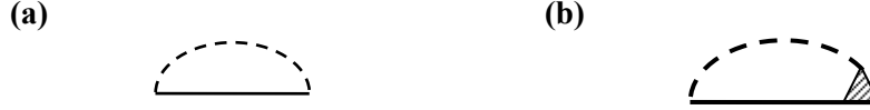
Fig. II.10.5 Corrections to the proper self-energy of the electron Green's function due to electron-phonon coupling: (a) the skeleton diagram for the lowest order correction; (b) the generalized diagram consisting of the vertex part.
