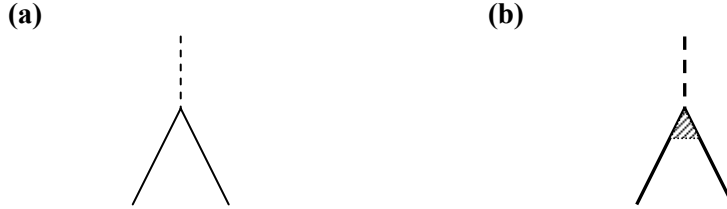
Fig. II.10.7 The Feynman diagrams associated with electron phonon interaction: (a) the first-order perturbation theory approximation; (b) the generalized expression containing all diagrams associated with the vertex part.
