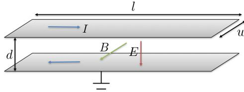
In a traveling wave that moves to the right, the current oscillates as
