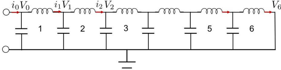
All the capacitors have the same capacitance  $C$ , and all the inductors have the same inductance  $L$  and no resistance. The bottom wire is grounded (has zero voltage). When we apply a harmonically oscillating signal from a signal generator through a coaxial cable to  $V_0$ , different oscillating voltages will be induced along the line in the steady state. That is if  $V_0(t) = V \cos \omega t$ , then  $V_j(t)$  has the form  $V_j(t) = A_j \cos \omega t + B_j \sin \omega t$ .
