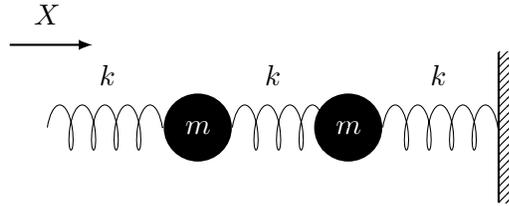
(a) Write down the equation of motion for the two masses. Write the equation in the matrix form and as an inhomogeneous second order differential equation.
