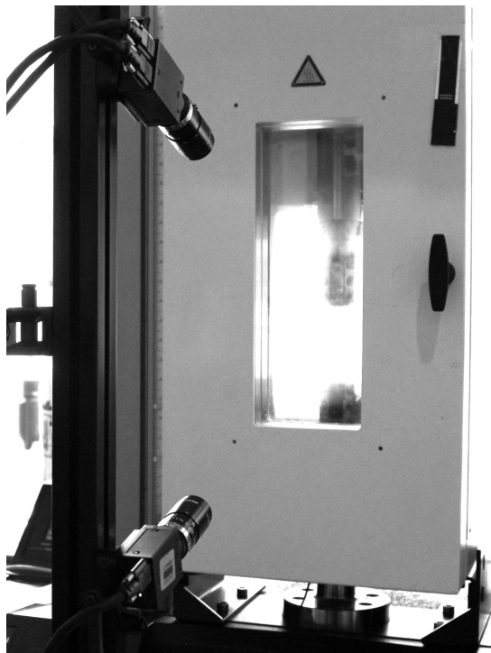
Fig. 7 Instron thermal chamber with DIC cameras.
