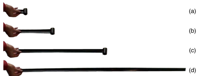
Fig. 11 Snapshots of the deployment of the tape spring with zero stowage time, with (a) t = 0.10 s, (b) t = 0.28 s, (c) t = 0.38 s, (d) t = 0.42 s
