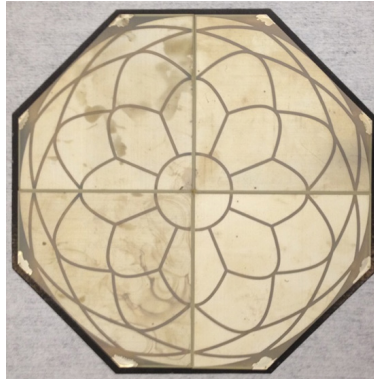
Figure 4. Backside of a 150 mm dia. CSM prototype containing four PZT-5A plates with a custom electrode pattern designed to correct for astigmatism-based errors.
