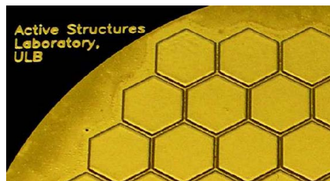
Figure 2. Silicon bimorph mirror with hexagonal PZT patches. 11
