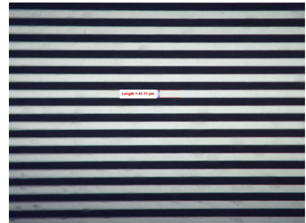
Encoder strip interval after bonding
