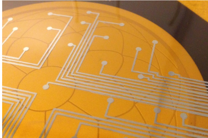
Figure 6. Backside of an active CFRP mirror after electrode routing layer integration.
