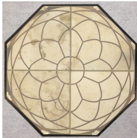
Figure 5. Backside of a 150 mm dia. active mirror prototype containing four PZT plates with a printed electrode pattern.
