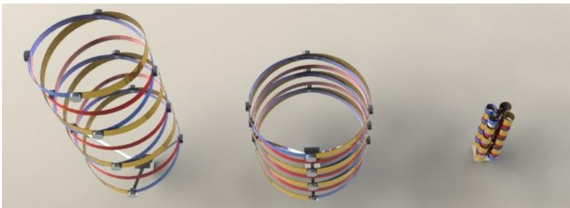
Figure 8. Helical pantograph concept shown fully deployed, axially compacted, and radially compacted.
