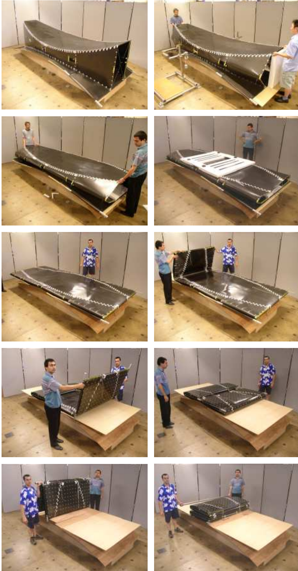
Figure 14: Packaging sequence, from top left to bottom right.
