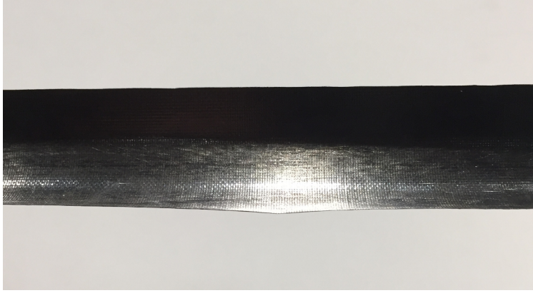
Figure 10. Kink appearing at a load of 0.027 N m (Sample 3).
