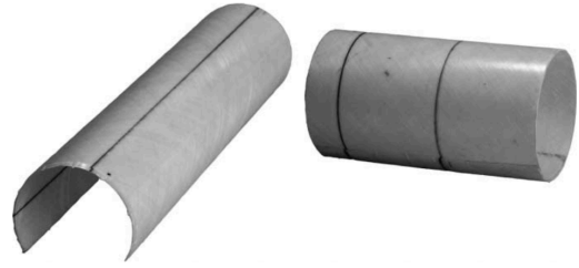
Fig. 1. Bistable tape springs in coiled and uncoiled configurations [1].
