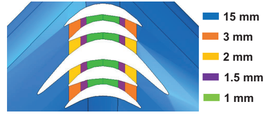
Figure 13. Sections of two-ply region simulated with lower stiffness and strength.
