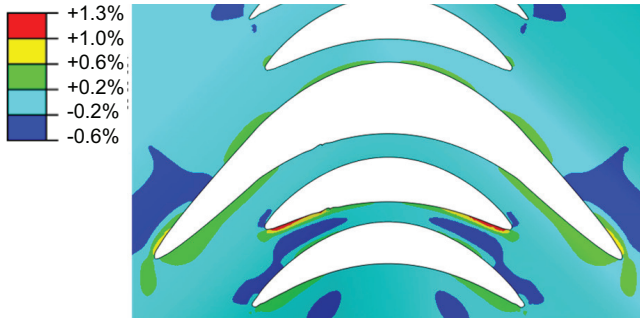
Figure 1. Contour plot of longitudinal strain \epsilon_{11} in center region of corner hinge with multiple cutouts. The shell has been folded 45^\circ and the strains are mapped on the deployed configuration.
