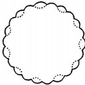
Figure 6: Cross-sections of dominant eigenmode of circular shell (solid and dashed arcs) and Aster shell (solid line) with R/t = 490 .
