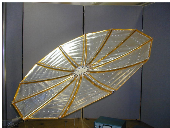
Figure 1: 1.5 m diameter model of CRTS reflector.
