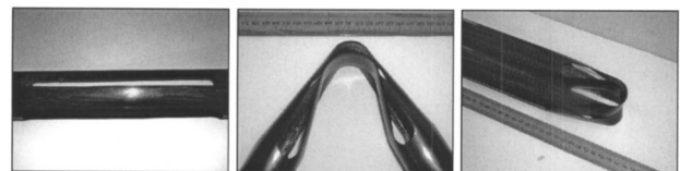
Fig. 1. Carbon fiber reinforced plastic tube hinge (unfolded, folded 110°, and folded 180°)
