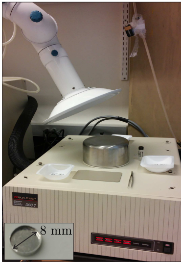
Figure 5. Left: Differential Scanning Calorimeter (DSC) employed in the resin cure kinetic modeling; the aluminum hermetic DSC pan containing 7-10 mg of resin is shown in the inset. Right: specific heat flow \bar{\Phi} = \Phi/w as a function of temperature during a DSC dynamic thermal scan performed at 10°C/min for an uncured sample. The glass transition temperature is at 53.09°C, while the exothermic peak occurs at 143.37°C. The dashed black line represents the baseline, necessary to calculate the amount of heat generated during cross-linking.
