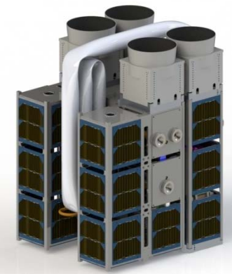
Fig. 3: AAReST launch configuration
