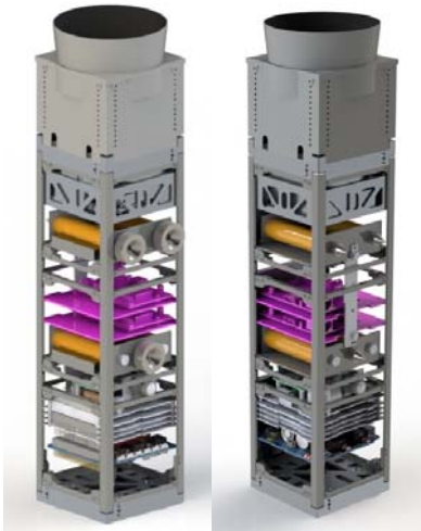
Fig. 15. MirrorSats showing the EM docking systems
