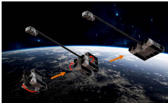
Fig. 4: AAReST concept demonstrating the launch configuration (left), initial imaging configuration (middle) and secondary imaging configuration (right)
