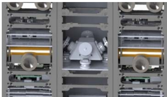
Fig. 22. View of the 4-wheel RWA in the CoreSat
