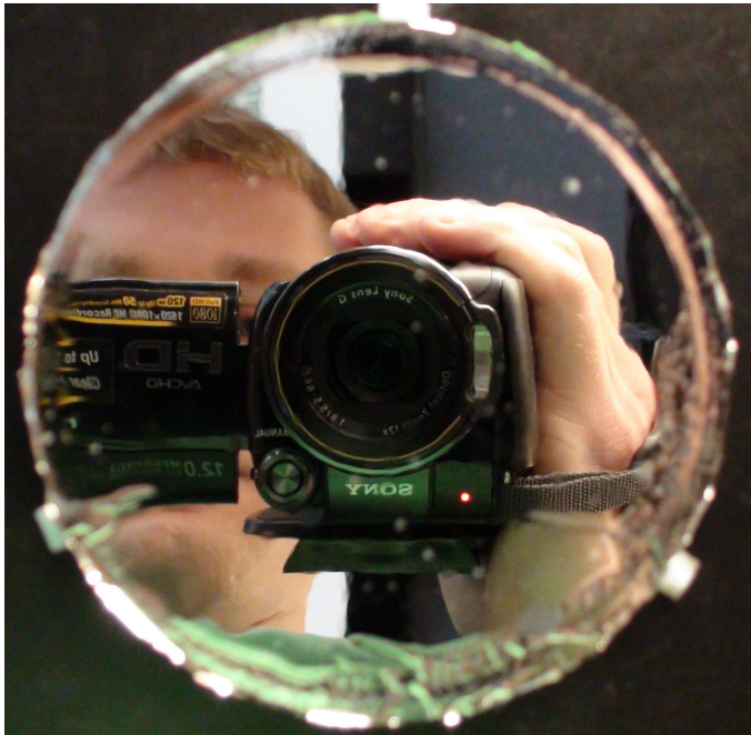
Figure 9. Film sample attached to a rim, showing the quality of the reflective front surface that can be achieved by replication from the wafer mold. Damage caused by peeling of the film stack from the silicon wafer can be seen around the edge.
