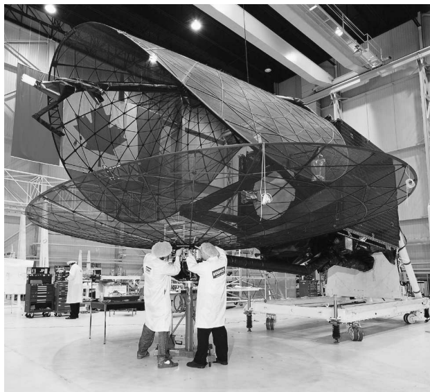
Figure 1. Spring back reflectors (one folded and one deployed) on MSAT-2 spacecraft, from reference 1.
