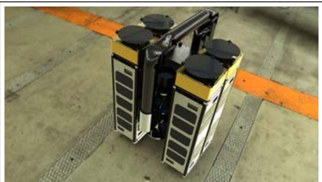
The latest concept for the AAReST spacecraft in the stowed configuration. Four small spacecraft with mirrors on top are shown attached to the center "nanosat," which holds the folded boom and optics package. The front two spacecraft
