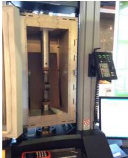
Characterize viscoelastic properties and perform accelerated aging tests
