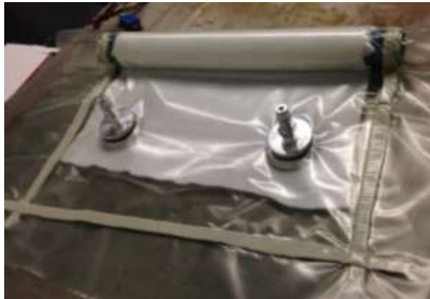
Manufacture hinges [ \pm 45_{AQ} / 0_{3CF} / 90_{CF} / \pm 45_{AQ} ]
