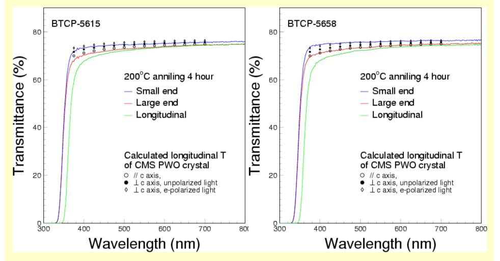
Some longitudinal non-uniformity in the transverse transmittance.
