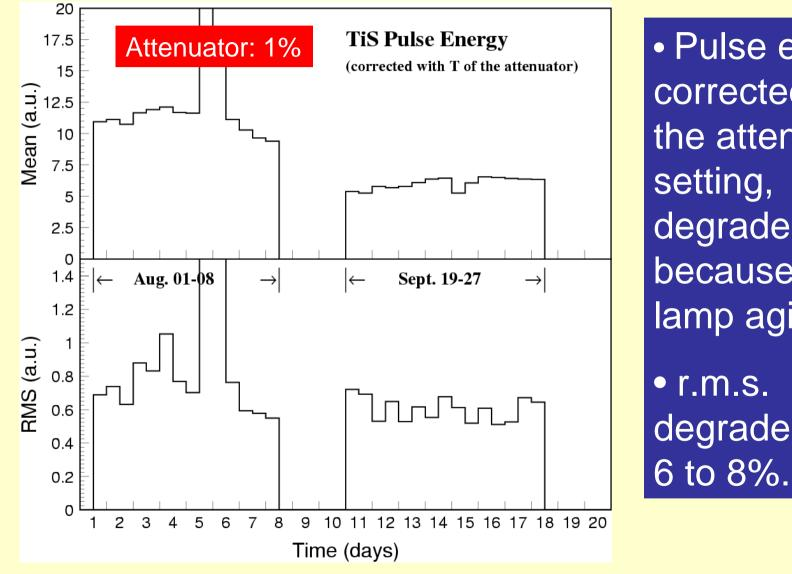
• Pulse energy, corrected by the attenuator setting, degraded because of lamp aging. • r.m.s. degraded from
