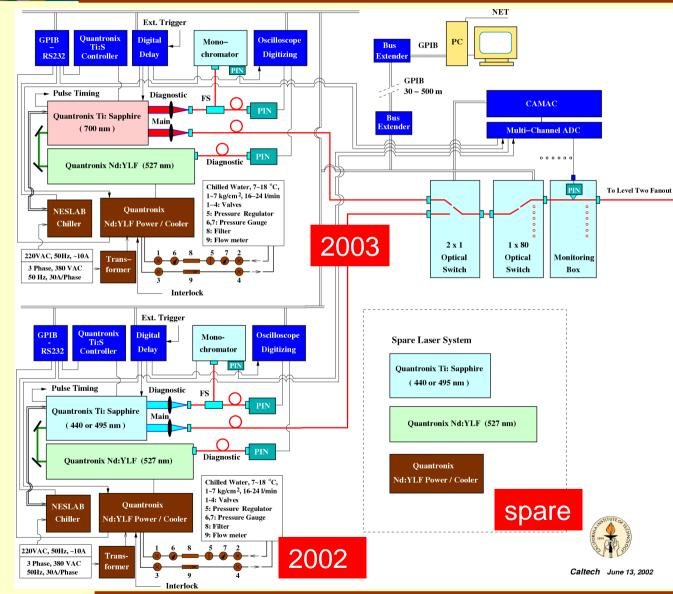
• Two laser systems: at 440/495 nm and 700/800 nm with own diagnostics on wavelength, pulse shape and intensity.
