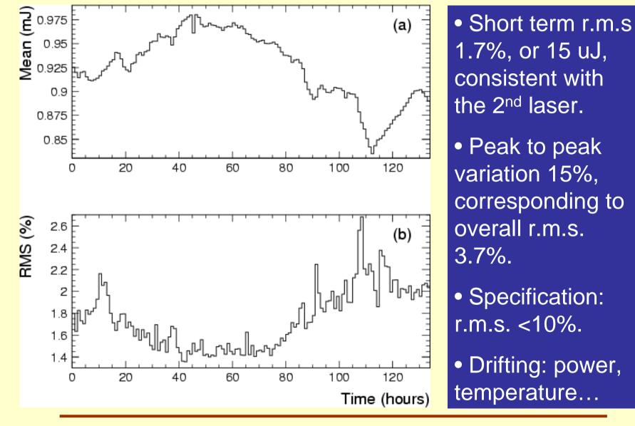
1.7%, or 15 uJ, consistent with the 2<sup>nd</sup> laser. • Peak to peak variation 15%, corresponding to overall r.m.s.
