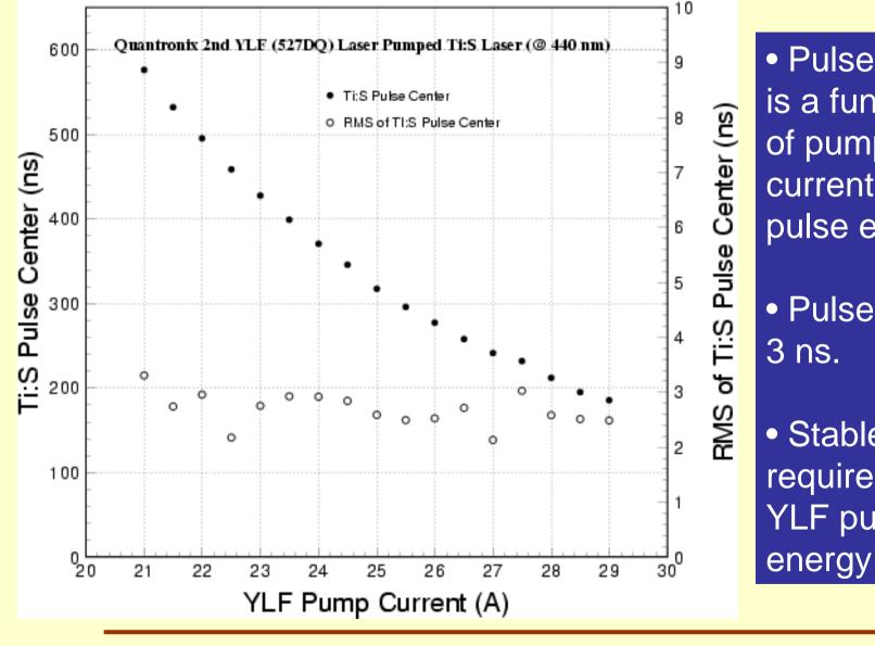
• Pulse timing is a function of pumping current or YLF pulse energy.
