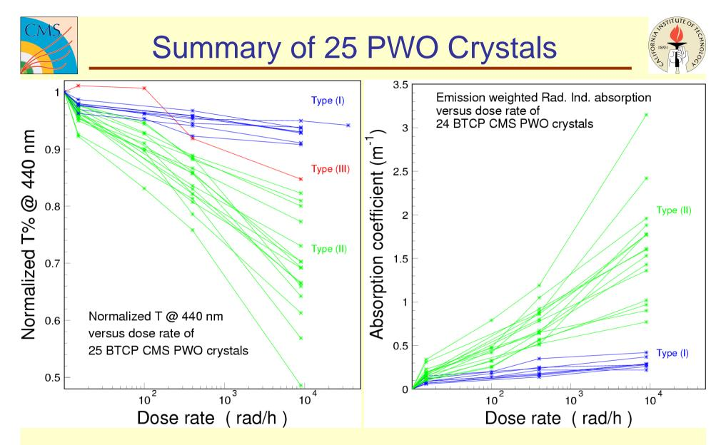
Radiation hard type I can be used for CMS endcaps, where 400 rad/h is expected. Relative hard type II crystals are for barrel (15 rad/h). Type III crystals are rejected.
