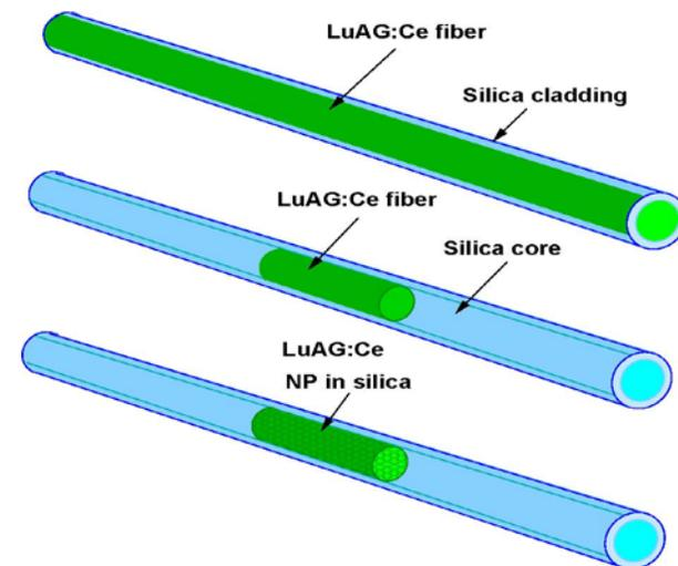
$\Phi 1 \times 40$  mm<sup>3</sup> SiC LuAG:Ce Ceramic LHPG fibers
