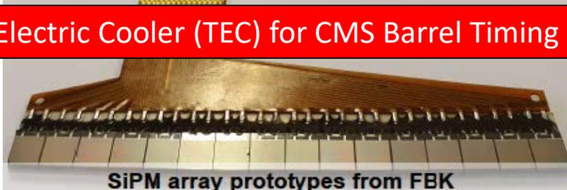
SiPM array prototypes from FBK
