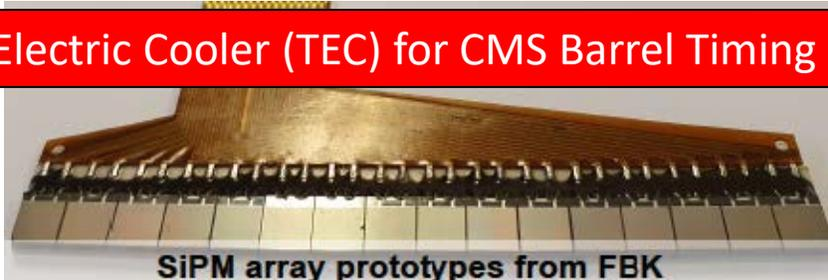
SiPM array prototypes from FBK
