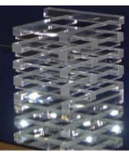
The HL-LHC and FCC-hh require fast and radiation hard calorimetry. The **RADiCAL** concept uses radiation hard LuAG:Ce ceramics as wavelength shifter for LYSO:Ce crystals for an ultra-compact, fast timing and longitudinally segmented shashlik calorimeter.
