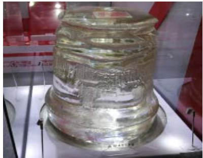
Large sapphire crystal of 400-450 kg
