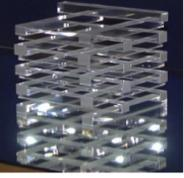
LYSO and BaF<sub>2</sub> are radiation hard up to  $8.3 \times 10^{15} \text{ n}_{\text{eq}}/\text{cm}^2$
