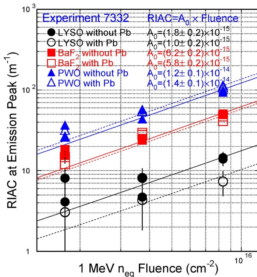
LYSO,  $\text{BaF}_2$  and PWO irradiated up to  $8 \times 10^{15} n_{eq}/\text{cm}^2$
