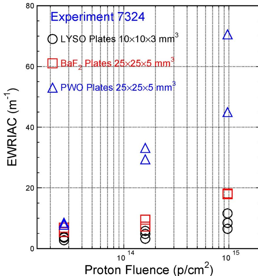
Excellent radiation hardness of LYSO and  $\text{BaF}_2$  up to  $10^{15} \text{ p}/\text{cm}^2$
