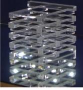
No damage observed in both transmittance and light output after 220 Mrad ionization dose and  $3 \times 10^{14}$  p/cm<sup>2</sup> of 800 MeV
