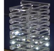
$N_{pe}/\text{channel}$  is 0.401 and 1.39 for 1 and 3 SiPM respectively
