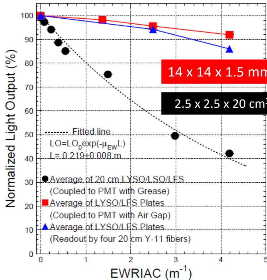
With EWRIAC of 3 m<sup>-1</sup>, LO losses in 14x14x1.5 mm plates and 20 cm long crystals are 5%/8% for direct/WLS readout and 50%
