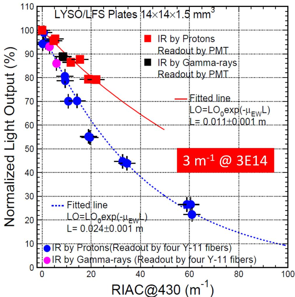
LO losses of 5% in  $14 \times 14 \times 1.5 \text{ mm}$  plates after  $3 \times 10^{14} \text{ p/cm}^2$
