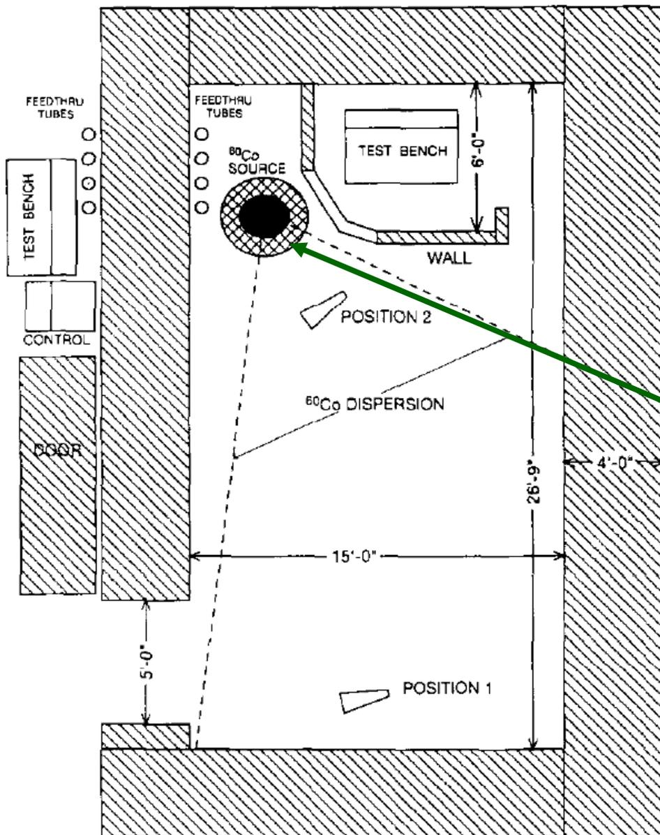
A group of high intensity  $^{60}\text{Co}$  sources provides a variable dose rate up to 1 Mrad/h in an opening throat of 10" x 10" x 13.5".
