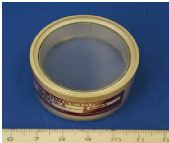
A sealed CeBr 3 crystal sample from Scionix Holland.
