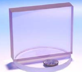
10x10x2 cm with 0.3 at. % Nd:YAG ceramic slab
