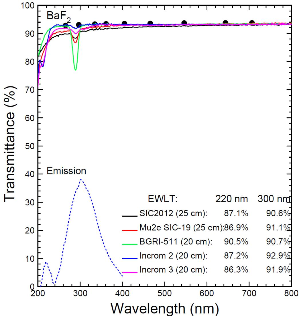
EWLT, or emission weighted longitudinal transmittance, is defined as:
