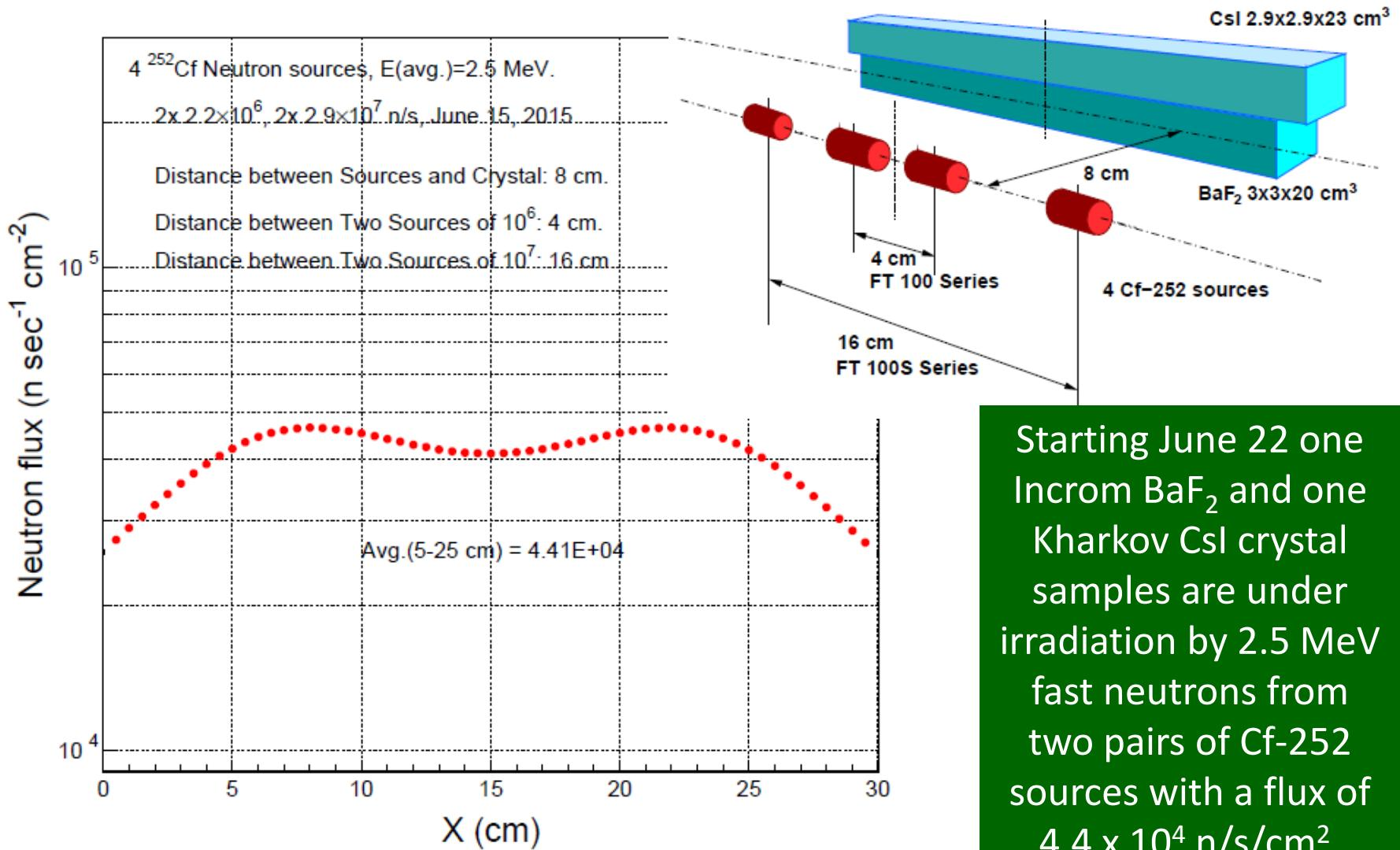
Starting June 22 one Incrom  $\text{BaF}_2$  and one Kharkov  $\text{CsI}$  crystal samples are under irradiation by 2.5 MeV fast neutrons from two pairs of  $\text{Cf-252}$  sources with a flux of  $4.4 \times 10^4 \text{ n/s/cm}^2$ .
