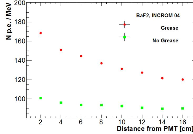
$$W \text{ grease} \rightarrow LY \sim (80 \div 100)N_{\text{p.e.}}/\text{MeV}, LRU \sim \pm(7 \div 11)\%$$
