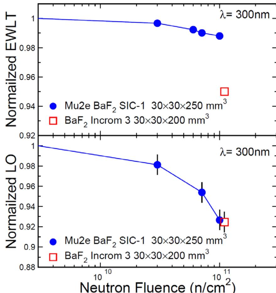
Caltech result is consistent with INFN result up to  $9 \times 10^{11} n/cm^2$
