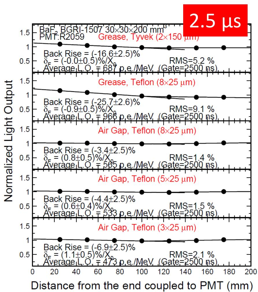
Result measured at Caltech is consistent with INFN data
