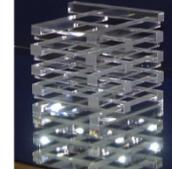
LSO/LYSO is a bright (200 times of PWO), fast (40 ns) and radiation hard crystal scintillator. The longitudinal non-uniformity issue caused by tapered crystal geometry, self-absorption and cerium segregation can be addressed by roughening one side surface. **The material is widely used in the medical industry. Existing mass production capability would help in crystal cost control.**
