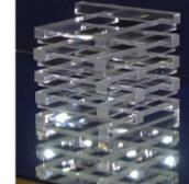
A Fermilab team (A. Para et al.) proposed a total absorption homogeneous hadronic calorimeter (HHCAL) detector concept to achieve good jet mass resolution by measuring both Cherenkov and Scintillation light.
