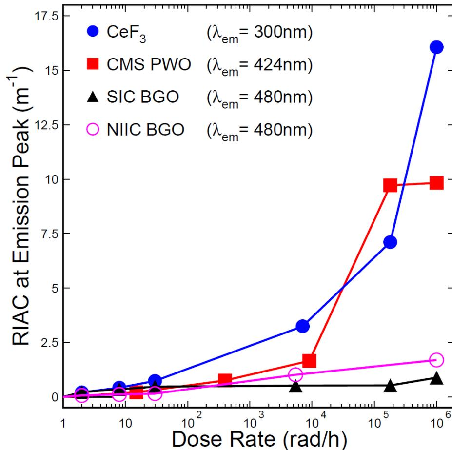
**BGO, LYSO and BaF<sub>2</sub> are radiation hard crystals**
