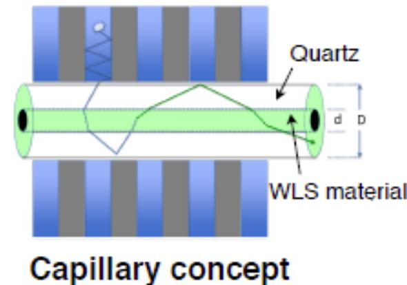
Replacement EM calorimeter using radiation tolerant crystal plates (LYSO/CeF<sub>3</sub>) interleaved with tungsten absorber. **Expected EM resolution: 10%/√E ⊕ 1%**
