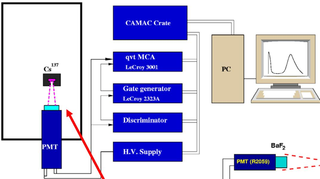
1) LYSO plates with Tyvek wrapping are readout directly by a R1306 PMT using a Cs-137  $\gamma$ -ray source.
