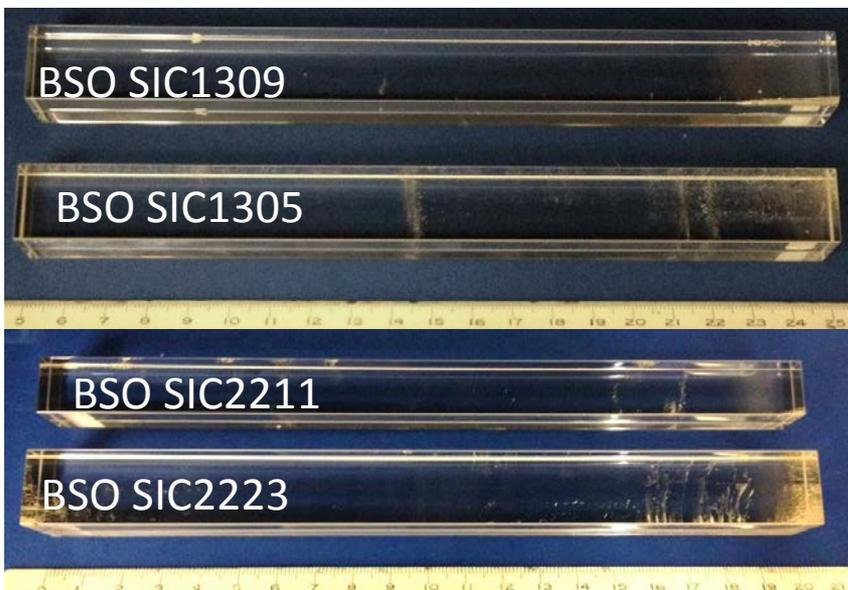
20 x 20 x 200 mm BSO crystals shows good optical and scintillation properties.
