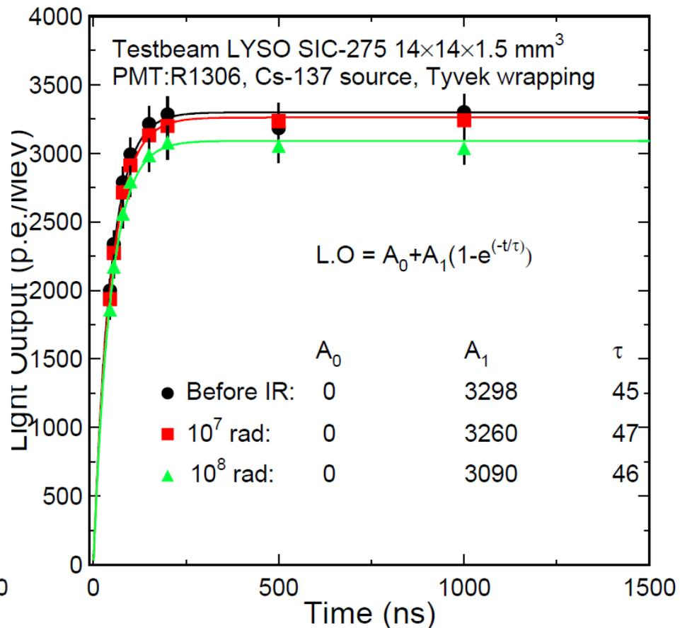
About 6% loss in light output is observed up to 100 Mrad
