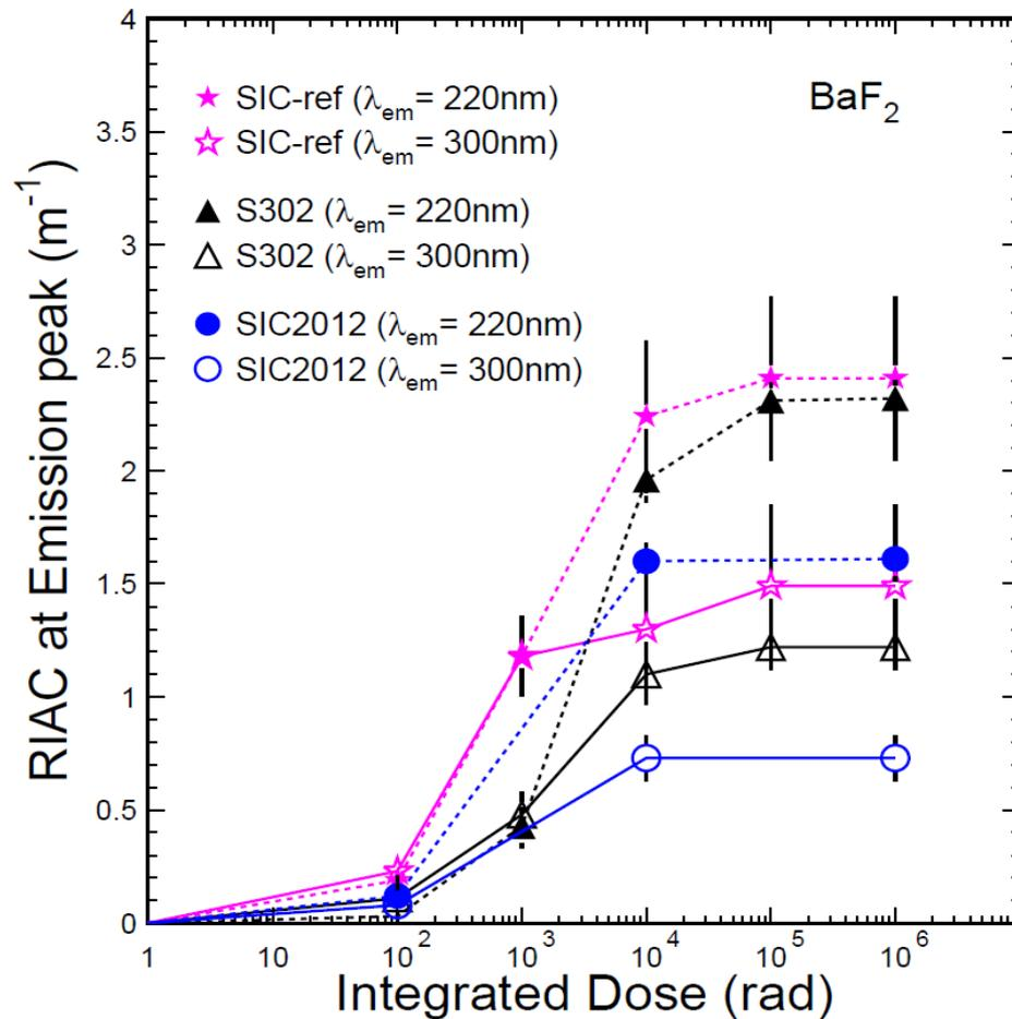
RIAC of mass produced BaF<sub>2</sub> may be controlled to less than  $1.6 \text{ m}^{-1}$
