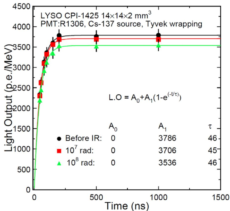
About 6/8% loss in light output is observed up to 100/200 Mrad
