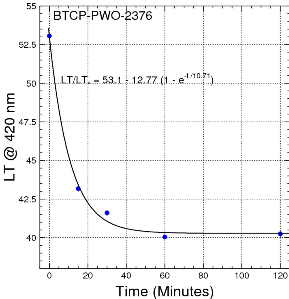
The time constant for the damage process @7,000 rad/h is about 10 minutes
