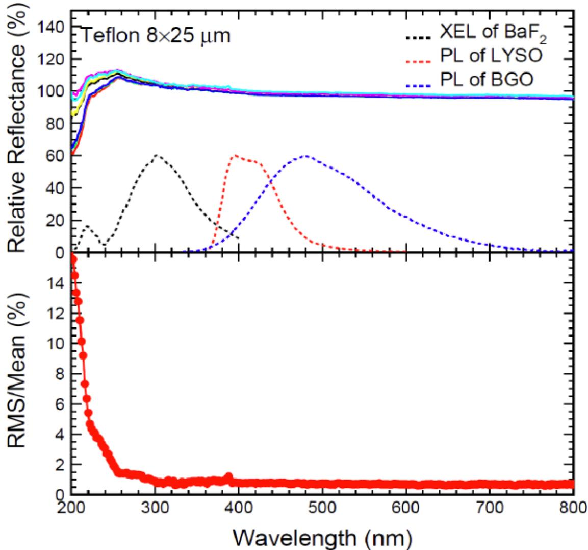
RMS values extracted from ten repeated measurements for 8 layers of Teflon films:
