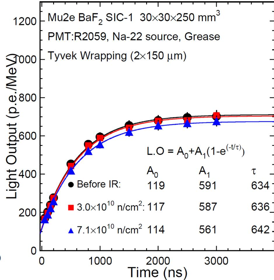
Up to  $7 \times 10^{10}$  n/cm<sup>2</sup> of fast neutron of 2.5 MeV
