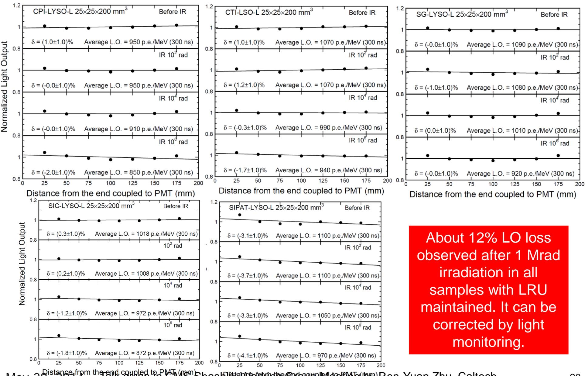
About 12% LO loss observed after 1 Mrad irradiation in all samples with LRU maintained. It can be corrected by light monitoring.
