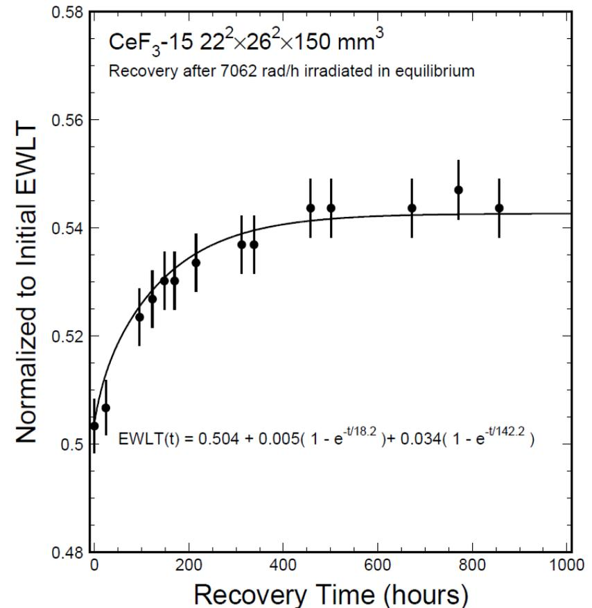
Consistent recovery time constants in two  $\text{CeF}_3$  samples from different vendors
