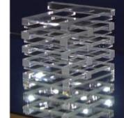
The smallest side surface of SIC-LYSO-L3 was roughened to  $R_a = 0.3$  at SIC via a two step process
