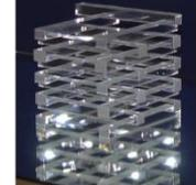
A LYSO matrix of 25 crystals was tested in May, 2011 at the beam test facility in Frascati. Crystals were uniformized by black painting of 15 mm at the small end of the smallest side surface
