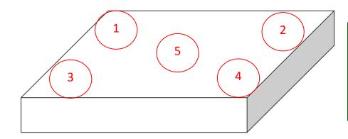
Good light response uniformity at a few percent level observed by injecting collimated <sup>137</sup>Cs source at five positions of the plate.
