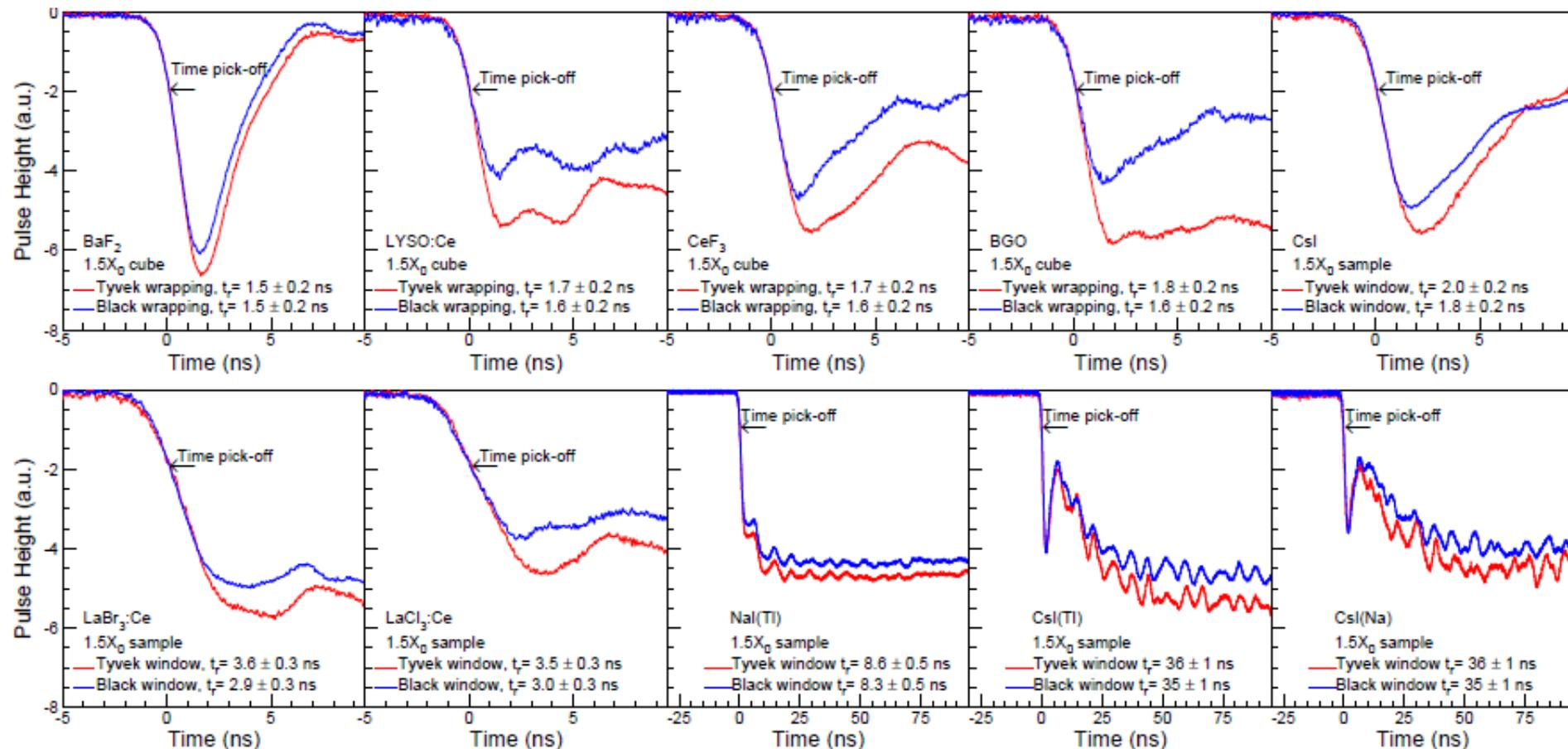
Measured rising time is dominated by photo-detector response, and is affected by light propagation in crystal.
