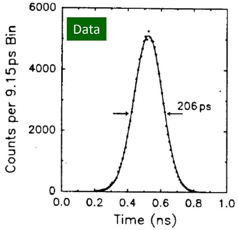
200 ps FWHM, or 60 ps  $\sigma_{\text{single}}$ , measured with BaF<sub>2</sub> & Hamamatsu R3377 PMT readout: a factor of three better than commercial system
