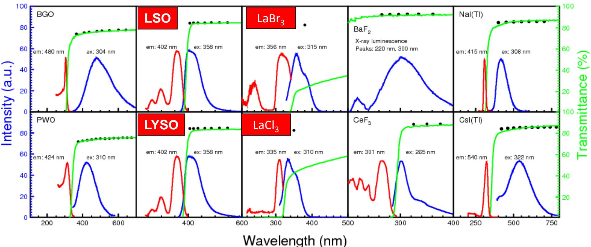
Poor transmittance indicates scattering centers: LaBr<sub>3</sub> and La Cl<sub>3</sub>
