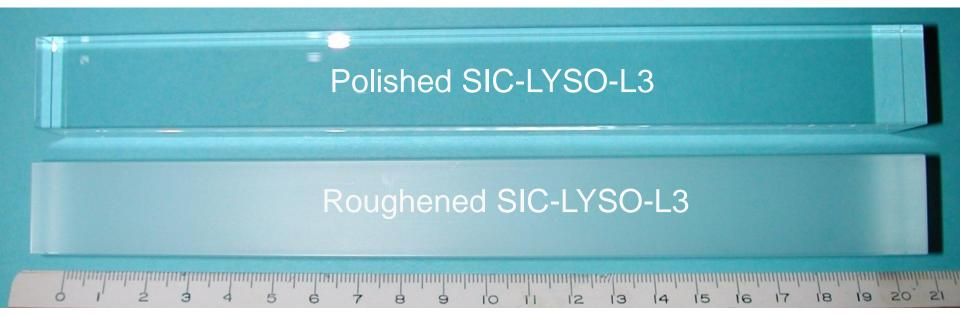
1st: lapped to Ra = 0.5 by using 11  $\mu$ m Al<sub>2</sub>O<sub>3</sub> powder for 10 min with 2.5 kg weight. 2nd: lapped to Ra = 0.3 by using 6.5  $\mu$ m SiC powder for 3 min with 1.5 kg weight.
