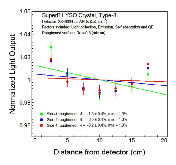
For the type-8 crystal with R<sub>a</sub>=0.3 roughening surface 4 (the smallest side surface) provides the best uniformity.
