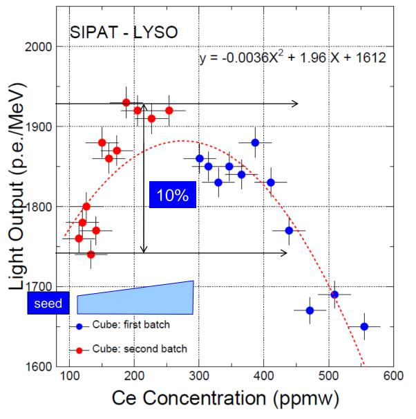
It is also known that cerium concentration along long LYSO crystals is not uniform, causing non-uniformity up to 10% at two ends, indicating up to 5% variation in  $\delta$ is possible because of cerium segregation.
